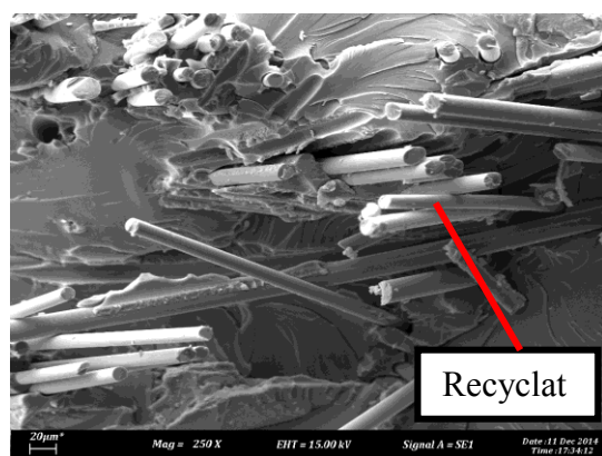
(c) SEM observations for rGFRP after bending test (250x zoom)
