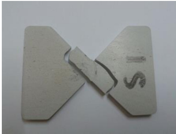
Figure 8: Brittle failure of ET2 specimen occurred at \pm 90^\circ
