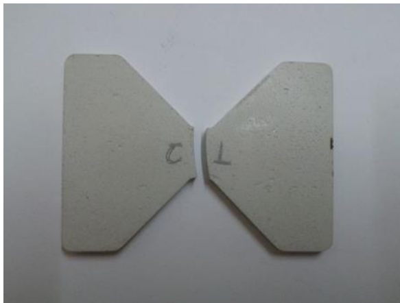
Figure 8: Brittle failure of ET2 specimen occurred at \pm 90^\circ
