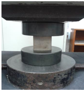
(a) Compressive strength testing
