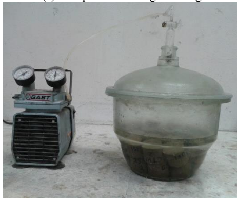
(c) Vacuum intrusion porosimetry testing
