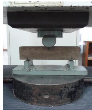
(b) Flexural strength testing
