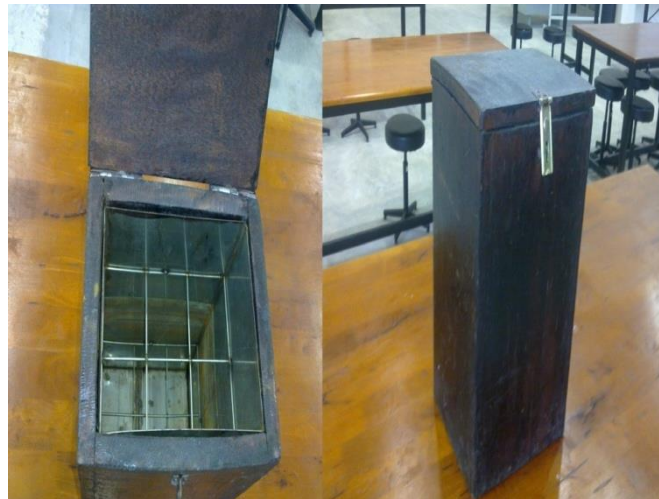
Figure 2: Constant-Load Stress Corrosion Cracking Test Chamber
