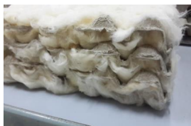
Figure 1: Sandwich Panel Partition for Egg Carton
