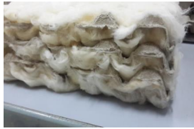
Figure 2: Complete Layered Sandwich panel aluminium cans partition walls
