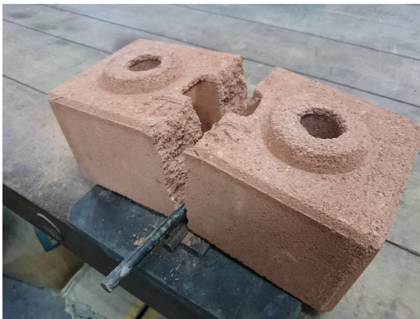
Figure 9: Failure of Splitting Tensile Test
