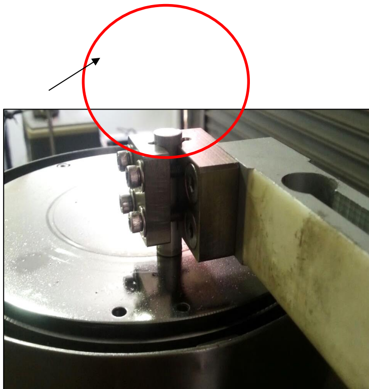
Figure 8: The location of the designed POD holder on the POD tribometer
