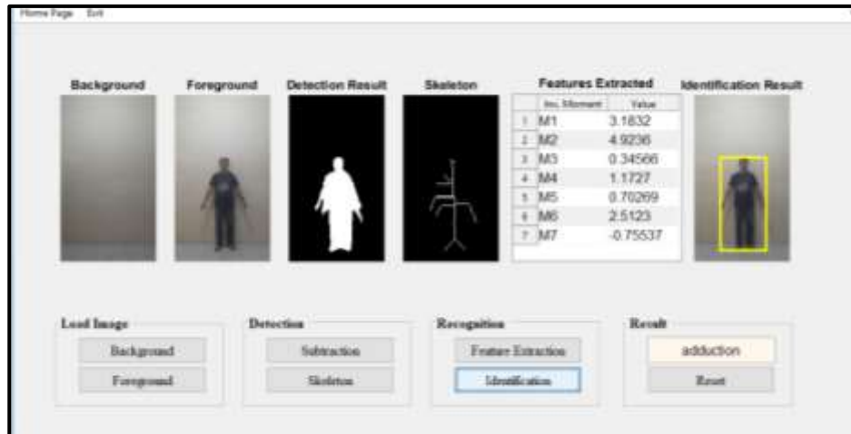
Figure 9 Recognition feature extraction with moment invariant
