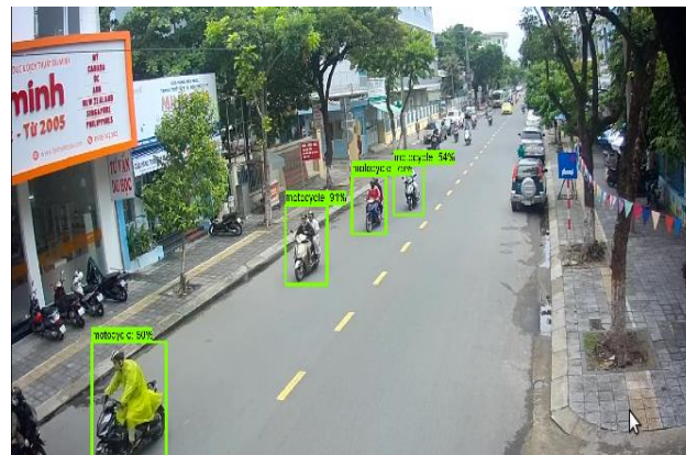
Figure 4: The result of motorcycle identification using video recorded by the camera.
